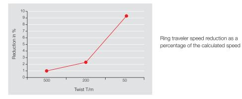
With low twist rates, the effective ring traveler speed is significantly lower than the calculated speed.
