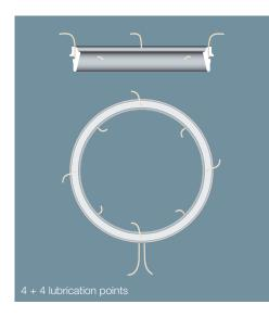
Spinning long staple fibers requires lubricated spinning rings.
