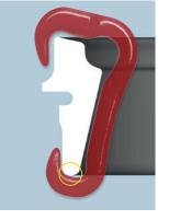
Excessive wear on foot tension is too low
