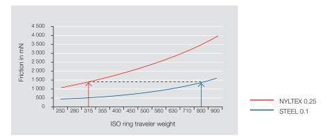
A NYLTEX ring traveler weight of 315 mg creates the same amount of friction as a STEEL ring traveler with a weight of 800 mg (the coefficient of friction may vary in practice due to lubrication, environment, etc).
