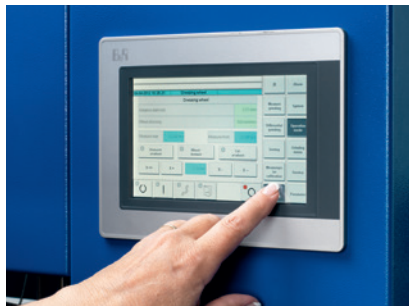
Machine is operated using the user-friendly touchscreen panel
