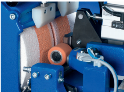
BERKOL high-performance grinding stone
